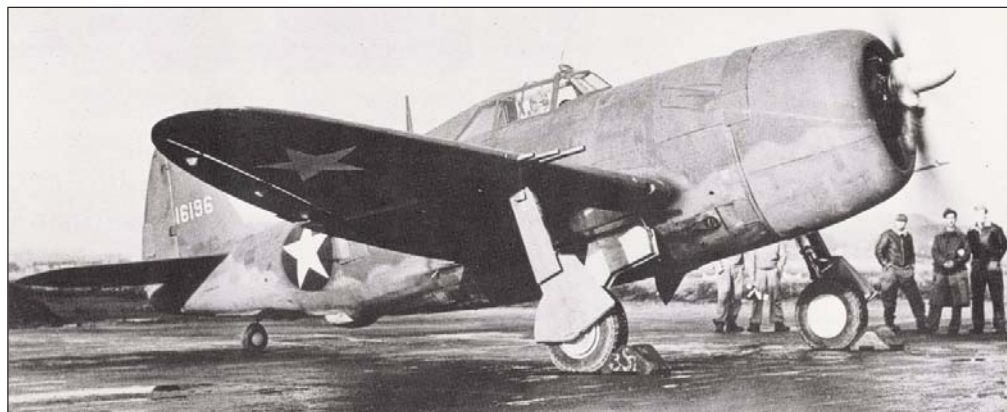
P-47D "Thunderbolt" weighed in at 7 tons with a 41 foot wingspan. It could fly at 430 MPH and with external fuel tanks it had a range of about 1,000 miles.
