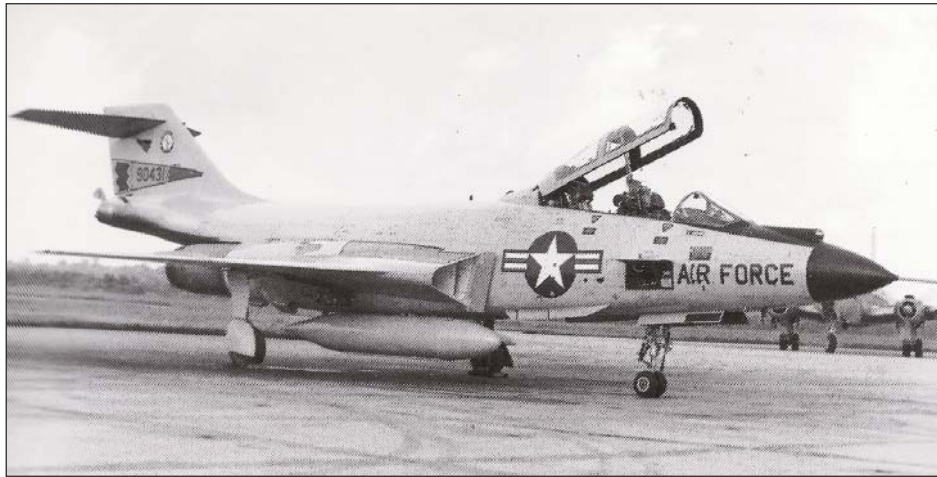
The McConnell F101B "Voodoo" had a swept wing span of less than 40 feet, but it could carry 2 external nuclear rockets as well as internal bombs or rockets to a height of 50,000 in under 6 minutes and then attack at 1100 MPH.
