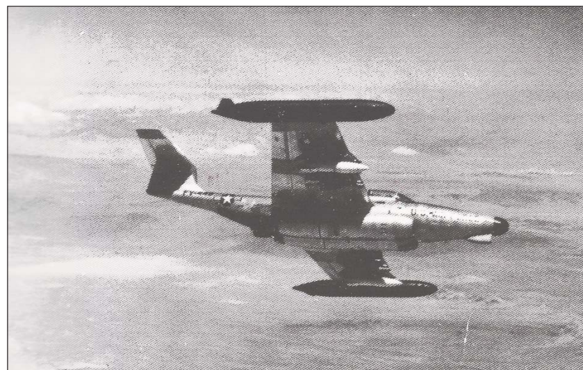
Northrop's F-89J "Scorpion" weighed in over 21 tons, with a wingspan of nearly 60 feet and a top speed of 635 MPH using its after burner. It was armed with rockets rather than guns, including the Genie nuclear rockets in its last version.
