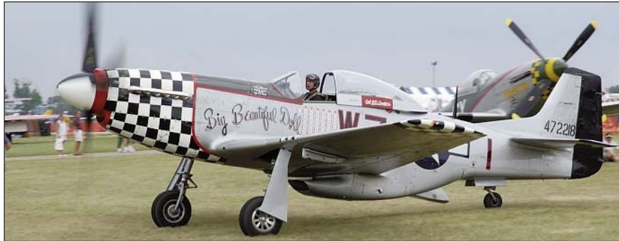
The P-51D “Mustang” flown by 78th FG commander, Col John D. Landers, showing his personal paint scheme Weighing about 6 tons, with a 37-foot wingspan this plane could fly about 1,000 miles with a top speed of 437 MPH.
