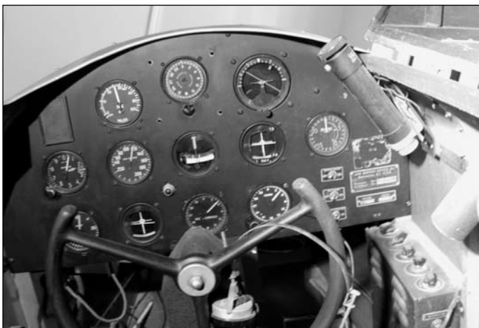
Instrument panel in cockpit of the Link trainer.
