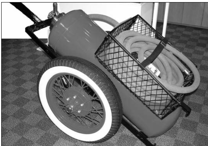
This picture is of one the hose cart's from the 1894 Fire Department. It had to be modified to a chemical cart and to be towed by a Model A. Notice the end will clamp on to the bumper. This cart also can be seen at the Novato Fire District Museum.
